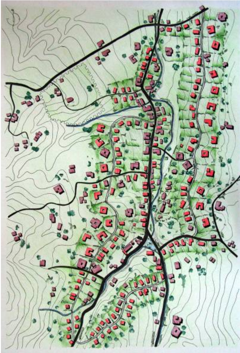
Image 5 - Proposed masterplan for Sohodol, one of the four villages surrounding Bran. Together with Bran these villages can take up all development in the foreseeable future and thus protect the character of the surrounding landscape. Image: ESUA.
