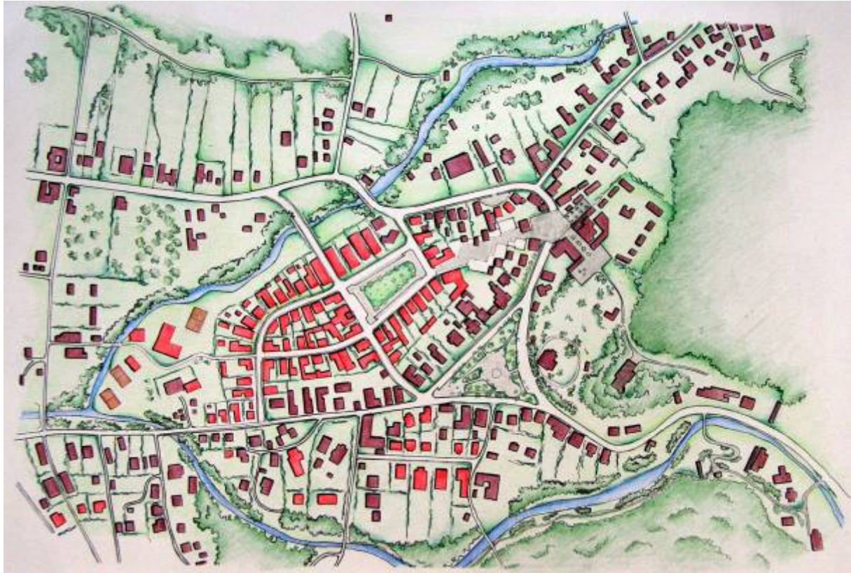
Image 4 – Proposed masterplan for the centre of Bran. Proposed new buildings are highlighted red, existing buildings are shown in brown. The extension of the town is defined by a proposed new civic square and a proposed new throughfare. Image: ESUA
